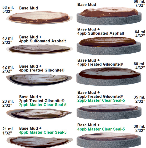
HPHT FILTRATION FILTER CAKES 250°F @ 500psi for 30 minutes
